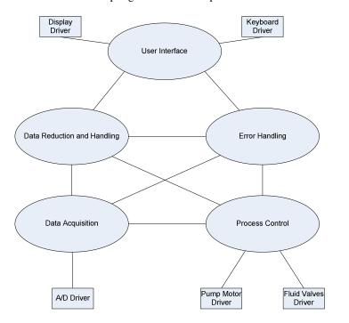
Each of the processes shall have further architectural decomposition and detailed design for each of the components, as requested by **clause 5.4 of IEC 62304**, but detailed design of each component is outside the scope of this example. For example, for the Data Acquisition process we could identify the following components:
