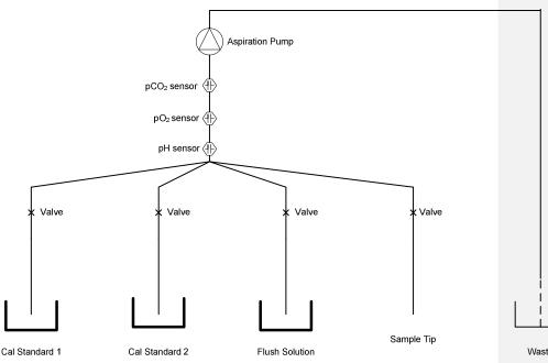
The software shall need to command the pump and the valves to aspirate the required solution until it is in contact with the sensors, activate the reading from the sensors, elaborate the data read from the sensors to present the results to the user, then command the pump and the valves to wash the lines with flush solution.
